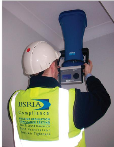
Powered flow hood, used for measuring flow rates from mechanical ventilation systems
